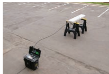
Fig. 3 Test set-up for antenna PIM measurement.
