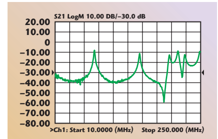
▲ Fig. 4 Broadband frequency response of a panel under test using the FSR test method.
